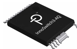
Figure 2. High Creepage, Safety-Compliant InSOP-24D Package.
