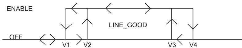
Figure 18. Line UVLO and OVLO Operation
