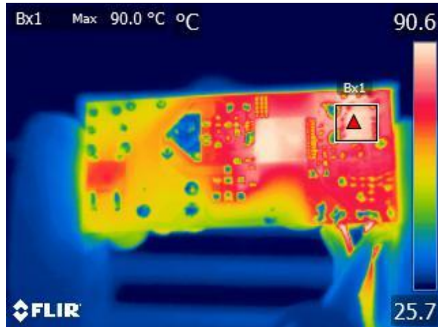
Figure 29 – Ambient = 25.7 °C. SR FET, Q3 = 90 °C.
