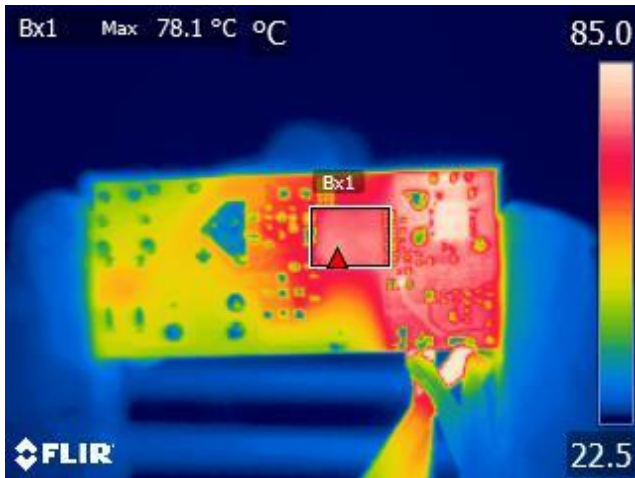
Figure 36 – Ambient = 22.5 °C. INN3279C, U1 = 78.1 °C.
