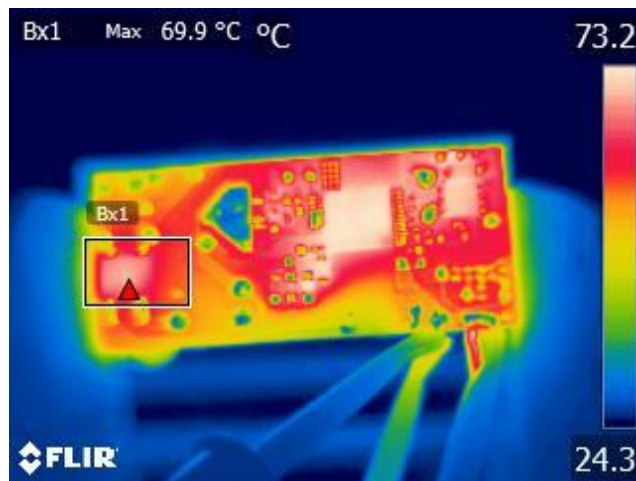
Figure 23 – Ambient = 24.3 °C. Bridge Diode, BR1 = 69.9 °C.
