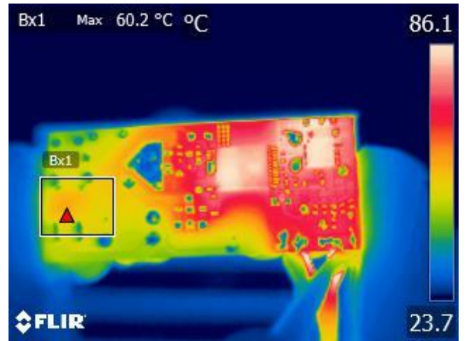
Figure 35 – Ambient = 23.7 °C. Bridge Diode, BR1 = 60.2 °C.
