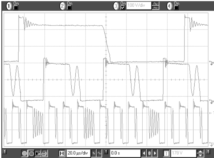
Figure 25. This plot gathers waveforms captured at three different operating points: 1 st Upper Plot: Free run, valley switching operation, P_{out} = 26 W. 2 nd Middle Plot: Min Toff clamps the switching frequency and selects the second valley. 3 rd Lowest Plot: The skip slices the second valley pattern and will further expand the burst as P_{out} goes low.
