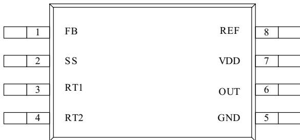
TSSOP-8 (Top View) PW Package
